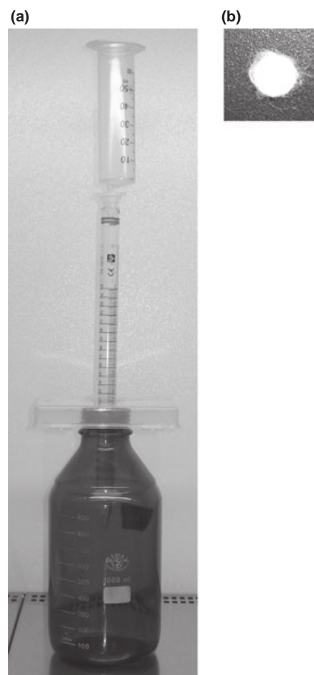
Figure 1 Description of system used to concentrate viruses. (a) System of filtration (b) dendrigrafts.
