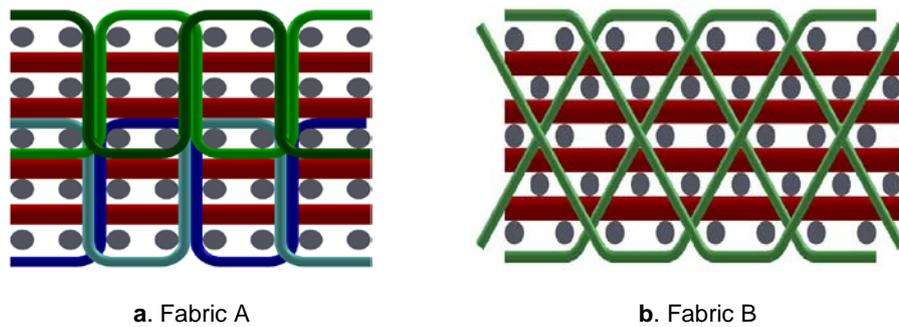
Figure 1. Weaving configuration of the two fabrics
