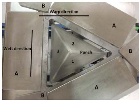
**Figure 2.** Forming device. A: rectangular blank holders. B: square blank holders. 1, 2, and 3: punch faces
