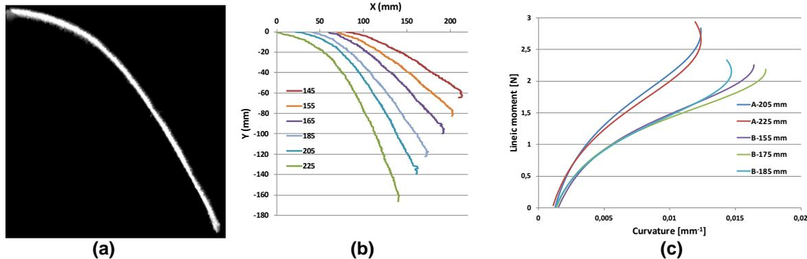
**Figure 5.** (a) Bending profile image (Fabric A, weft direction, bending length 215mm, additional weight 152 g). (b) Extracted bending profiles for different bending length (Fabric A, weft direction, additional weight 152 g). (c) Reconstructed moment-curvature curve of the 2 fabrics in the weft direction.
