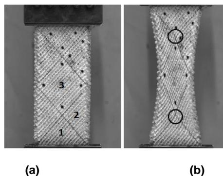
**Figure 4.** (a) Position of the different zones in a sample before testing. (b) Localization of the deformation of zones 1 during testing
