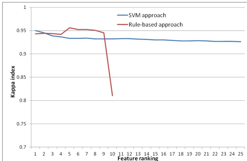
Figure 2. Mean Kappa indices computed based on SVM and rule-based approaches. The x-axis lists the features ranked according to the SVM-RFE approach or the Jeffries-Matusita distance (see table 1).
