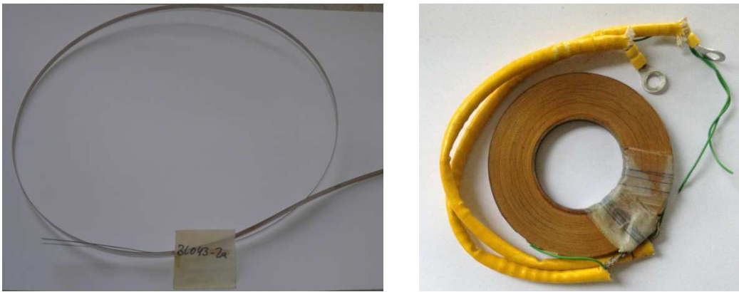
Fig. 3: Sample of superconducting wire (BSCCO2212) and superconducting coil picture used in the experiment
