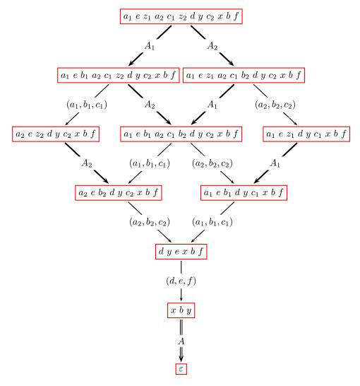
Fig. 3.4: Behavior graph of the block  $A = \text{and}(A_1, A_2)$ .
