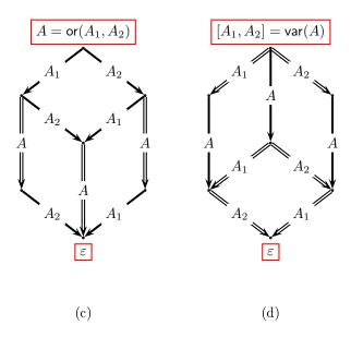
Fig. 3.7: Abstract representations of the blocks copy, and, or, and var, obtained from each behavior graph (Figures 3.3, 3.4, 3.5, and 3.6) by contracting arcs corresponding to internal triples, and keeping only the arcs corresponding to variables. We see, for each block, which output variables are activable, depending on which variables have been activated.
