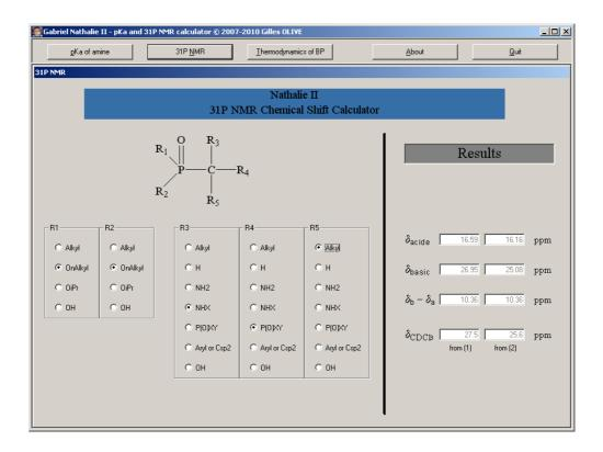
Fig. 2: Screen of GN2 for calculating <sup>31</sup>P NMR chemical shift values of phosphorylated compounds.<sup>3</sup>
