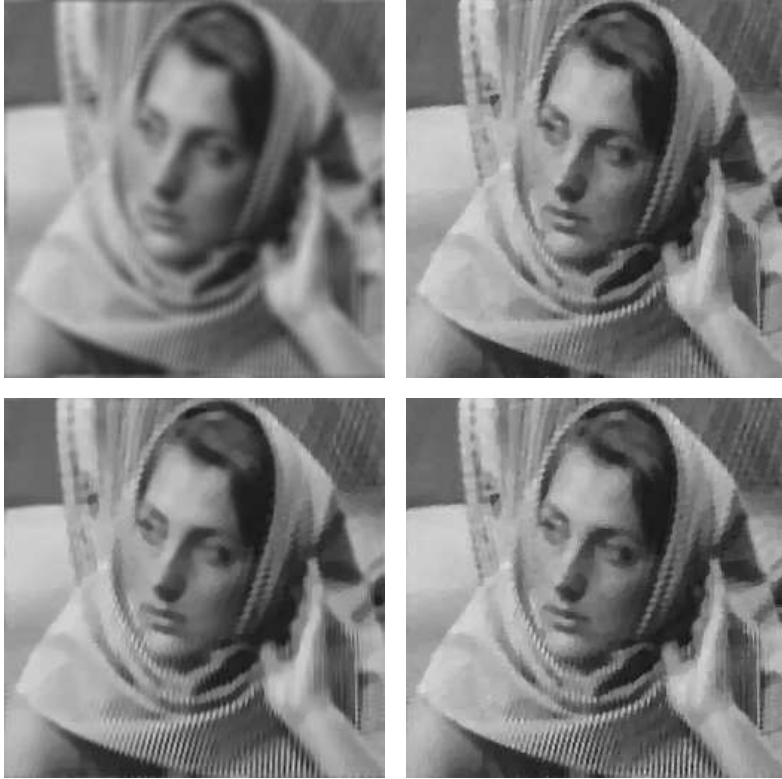
FIGURE 9. Restoration from uniform blur. Top, left: blurred image; Top, right: ROF model (522 iterations, CPU time=4.6s, PSNR=24.73dB); Bottom, left: LM model (1978 iterations, CPU time=1991s, PSNR=25.49dB); Bottom, right: Proposed model (1083 iterations, CPU time=968s, PSNR= 25.75dB).
