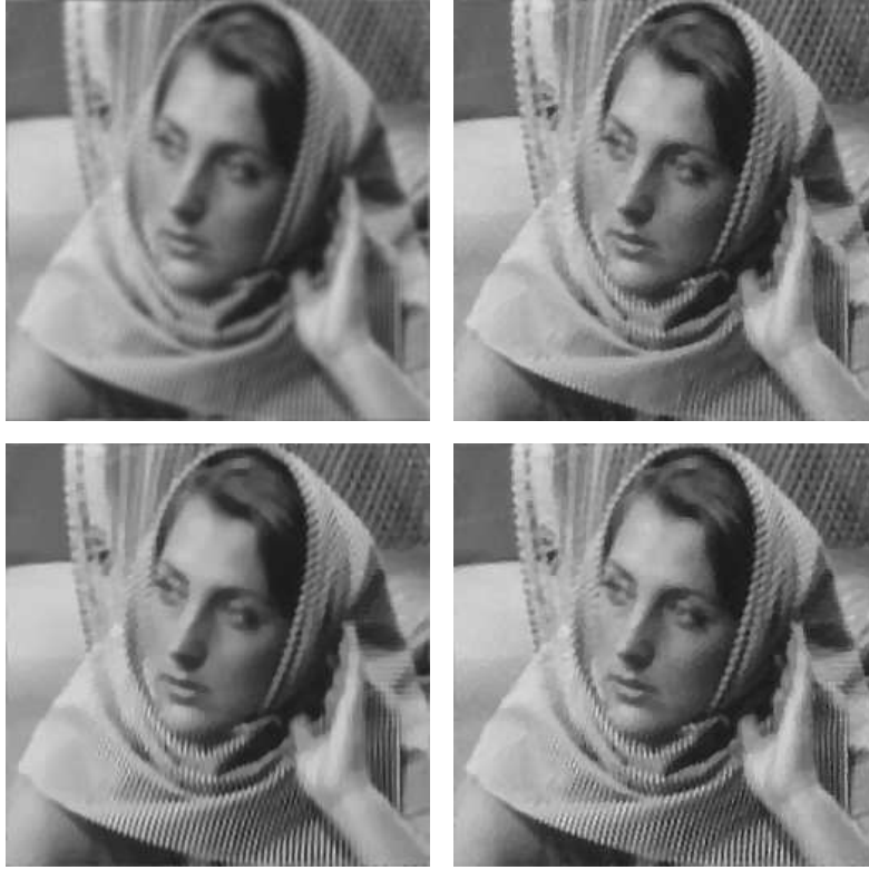
FIGURE 8. Restoration from Gaussian blur. Top, left: blurred image; Top, right: ROF model (452 iterations, CPU time=4.0s, PSNR=25.52dB); Bottom, left: LM model (1602 iterations, CPU time=1639s, PSNR=27.16dB); Bottom, right: Proposed model (966 iterations, CPU time=861s, PSNR= 27.43dB).
