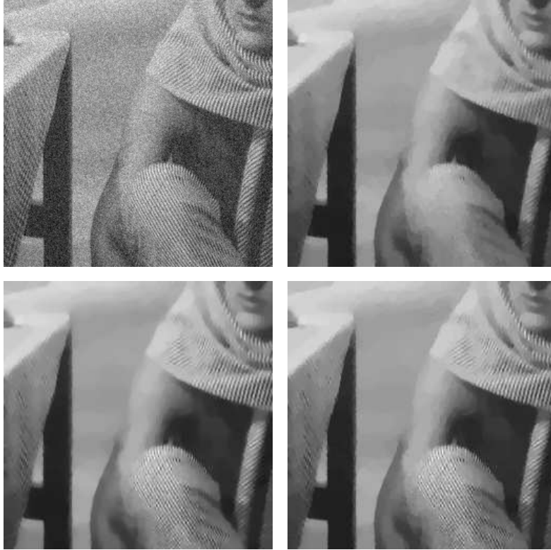
FIGURE 2. Denoising of a gray-level image. Top, left: noisy image; Top, right: ROF Model (787 iterations, CPU time = 3.9s, PSNR = 24.75dB); Bottom, left: LM Model (1456 iterations, CPU time = 1434s, PSNR = 26.09dB); Bottom, right: our model (281 iterations, CPU time = 241s, PSNR = 26.19dB).
