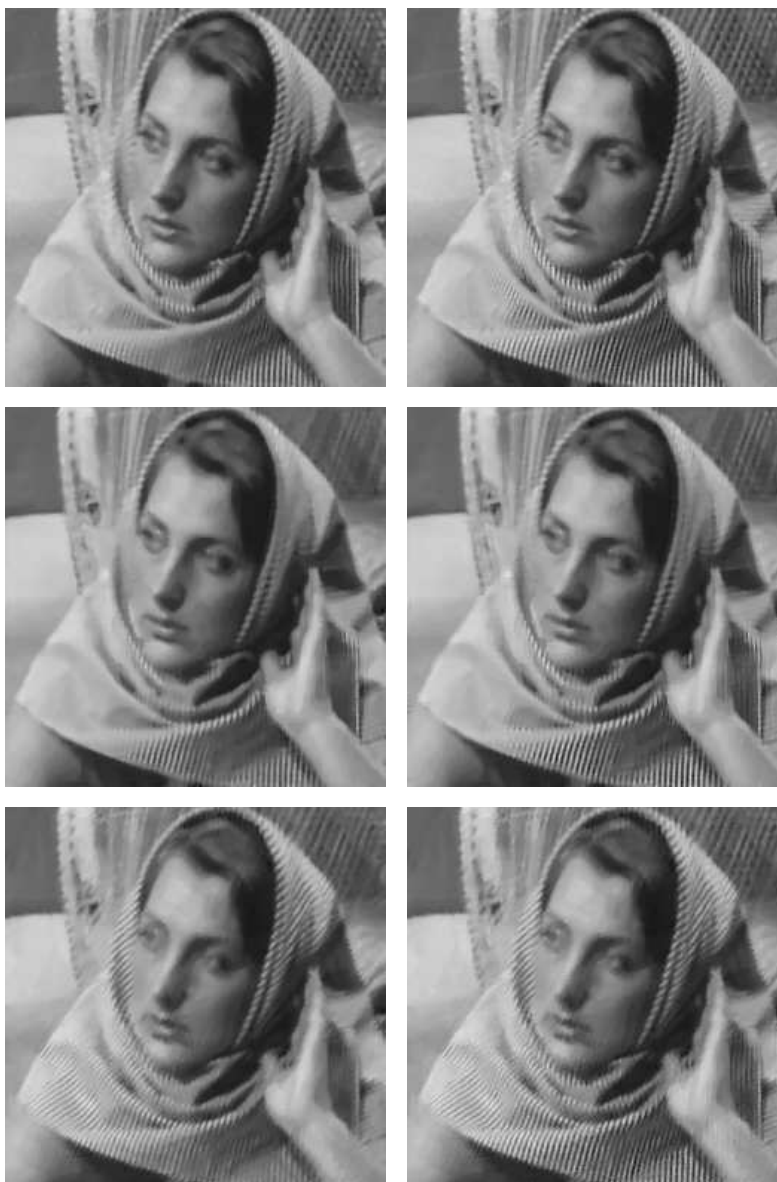
FIGURE 16. Results of image deblurring based on NLTV regularization. Left column: classical NLTV deblurring; Right column: proposed model combined with NLTV. From top to bottom: Gaussian blur (PSNR=26.44dB, 28.11dB), uniform blur (PSNR=25.48dB, 26.16dB), and motion blur (PSNR=25.79dB, 27.50dB).
