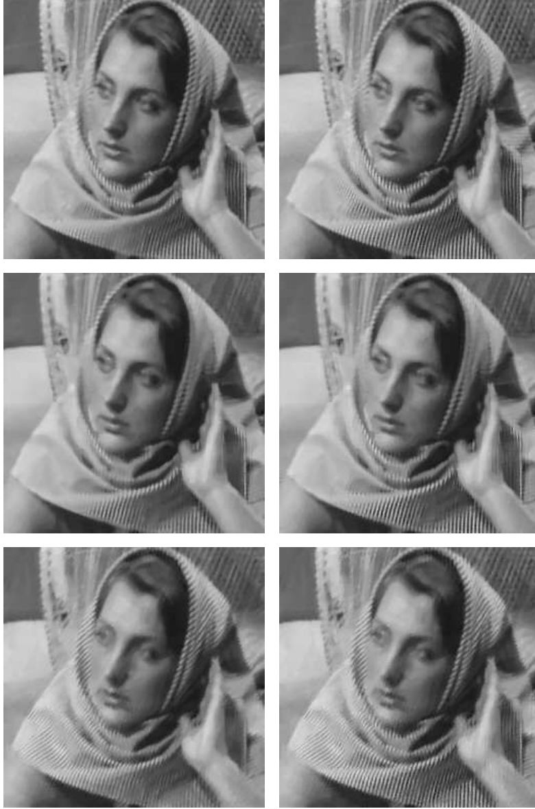
FIGURE 15. Results of image deblurring based on NLTV regularization. Left column: classical NLTV deblurring; Right column: proposed model combined with NLTV. From top to bottom: Gaussian blur (PSNR=26.44dB, 28.11dB), uniform blur (PSNR=25.48dB, 26.16dB), and motion blur (PSNR=25.79dB, 27.50dB).
