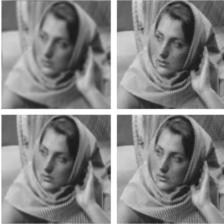
FIGURE 8. Restoration from uniform blur. Top, left: blurred image; Top, right: ROF model (522 iterations, CPU time=4.6s, PSNR=24.73dB); Bottom, left: LM model (1978 iterations, CPU time=1991s, PSNR=25.49dB); Bottom, right: Proposed model (1083 iterations, CPU time=968s, PSNR= 25.75dB).
