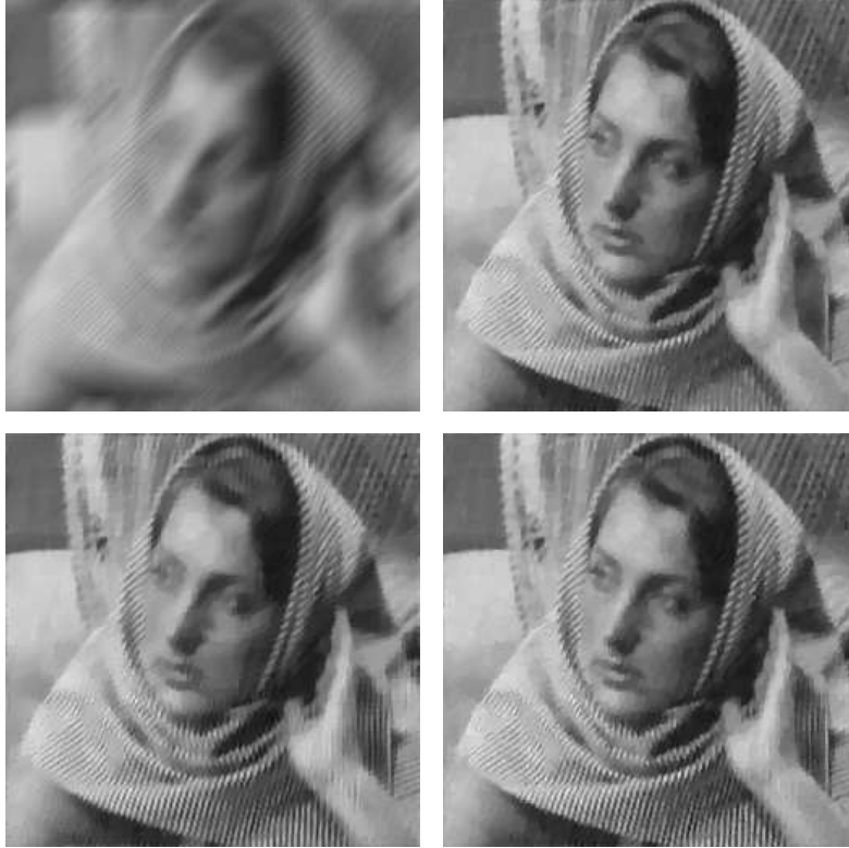
FIGURE 9. Restoration from motion blur. Top, left: blurred image; Top, right: ROF model (806 iterations, CPU time=8.1s, PSNR=25.58dB); Bottom, left: LM model (3348 iterations, CPU time=3402s, PSNR=26.21dB); Bottom, right: Proposed model (1546 iterations, CPU time=1382s, PSNR= 27.14dB).
