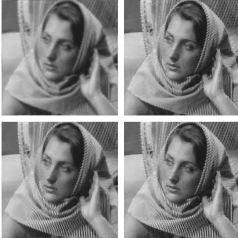
FIGURE 7. Restoration from Gaussian blur. Top, left: blurred image; Top, right: ROF model (452 iterations, CPU time=4.0s, PSNR=25.52dB); Bottom, left: LM model (1602 iterations, CPU time=1639s, PSNR=27.16dB); Bottom, right: Proposed model (966 iterations, CPU time=861s, PSNR= 27.43dB).
