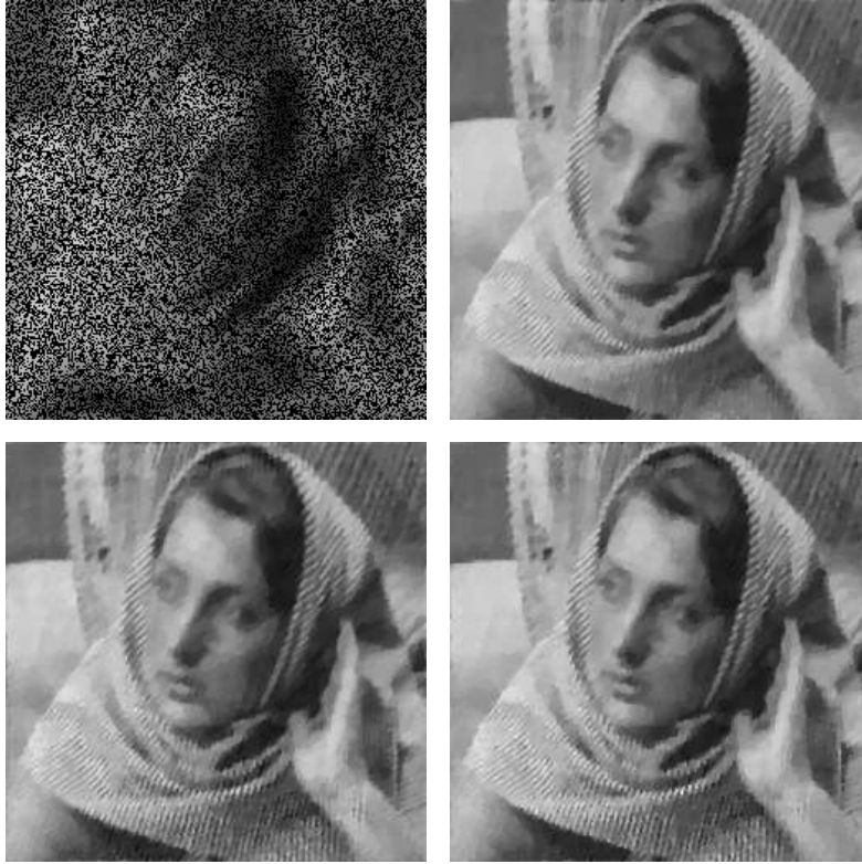
FIGURE 11. Image inpainting with randomly missing pixels. Top, left: corrupted image; Top, right: ROF model (993 iterations, CPU time=142s, PSNR=24.29dB); Bottom, left: LM model (2449 iterations, CPU time=2477s, PSNR=24.63dB); Bottom, right: Proposed model (1856 iterations, CPU time=2084s, PSNR=25.06dB).
