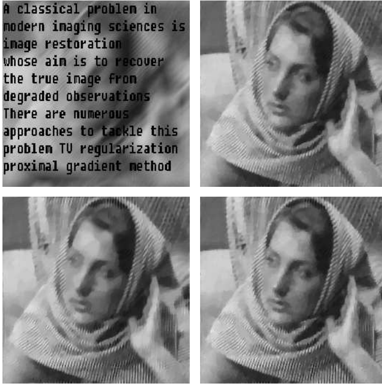
FIGURE 12. Image inpainting with structured missing pixels (superimposed text). Top, left: corrupted image; Top, right: ROF model (925 iterations, CPU time=151s, PSNR=25.06dB); Bottom, left: LM model (2721 iterations, CPU time=2803s, PSNR=25.30dB); Bottom, right: Proposed model (1388 iterations, CPU time=1546s, PSNR=26.20dB).
