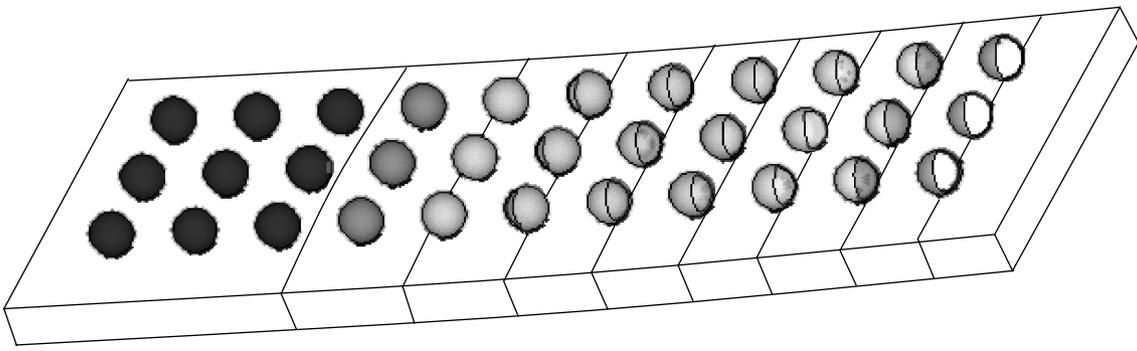
**Fig. 2.** The first bending mode of oscillations in the elastic plate.
