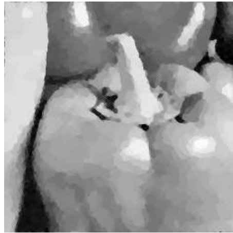
Total variation regularization SNR = 22.1 dB - SSIM = 0.69
