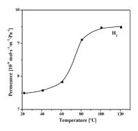
**Fig. 5**  $H_2$  permeance for a SIM-1 membrane as a function of the temperature.
