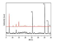
**Fig. 2** XRD patterns of (a) alumina-supported SIM-1 and (b) as-synthesized SIM-1. Reflections marked by \* correspond to the alumina support.
