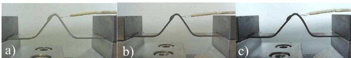
Fig. 13. Evolution of the specimen geometry during thermal fatigue tests on welded sample 8, (a) before testing, (b) after 2000 cycles, (c) at the end of the test.
