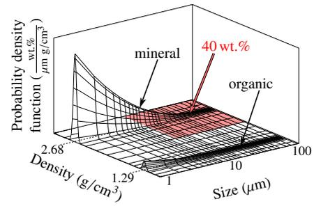
Figure 9: Washability of a sample of dredged sediment
