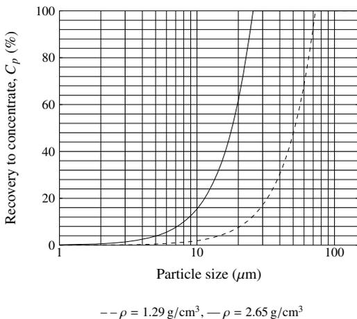
Figure 12: Predicted partition curves of a sample sediment with a Falcon L40 operating at  $0.18 Q^{-1}\omega^2 / (Q_0^{-1}\omega_0^2)$ , feed solid fraction being 21 wt.%.
