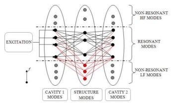
FIGURE 3. Modal interaction scheme of the sound transmission below the critical frequency.
