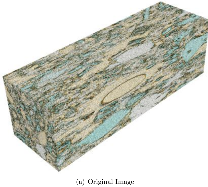
Figure 5.3: 3D X-ray stack of Tuffeau
