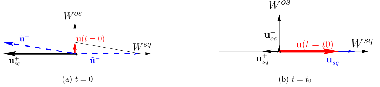
Figure 2: Sketch illustrating transient growth of an OS perturbation \mathbf{u} . \tilde{\mathbf{u}}^+ and \tilde{\mathbf{u}}^- are the eigenvectors, \mathbf{u}_{os} and \mathbf{u}_{sq} the projections on W_{mp}^{os} and W_{mp}^{sq} :
