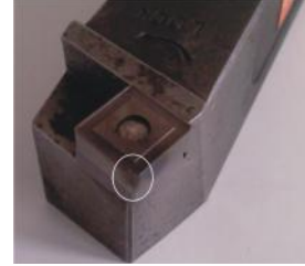
Figure 5. worn cutting tool
