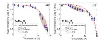
FIG. 3 (color). Temperature variation of the large gap  $\Delta_1(T)$  in (a) SnMo<sub>6</sub>S<sub>8</sub> and (b) PbMo<sub>6</sub>S<sub>8</sub>, measured by STS. The gap value was determined by fitting spectra acquired on a flat terrace (i.e., with a negligible  $\Delta_2$  component) using a BCS single-band anisotropic *s*-wave model.
