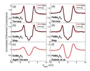
FIG. 2 (color). (a)–(c) SnMo<sub>6</sub>S<sub>8</sub> spectra and fits: T=0.4 K,  $R_T=0.03$  G $\Omega$ . (d)–(e) PbMo<sub>6</sub>S<sub>8</sub> spectra and fits: T=0.5 K,  $R_T=0.015$  G $\Omega$ . (f) PbMo<sub>6</sub>S<sub>8</sub> spectrum from [19]: T=1.9 K,  $R_T=0.025$  G $\Omega$ . See the text for details and Table I for fit parameters.  $2\Delta_1/k_BT_c$  in PbMo<sub>6</sub>S<sub>8</sub> is similar to data from [26].
