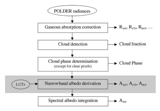
**Figure 1.** Diagram of the POLDER "ERB, water vapor, and clouds" level 2 processing line (ERB is Earth Radiation Budget). Only the part useful for the derivation of narrowband and broadband albedos is reported here. Object of the present paper is shaded in gray.
