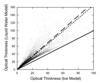
**Figure 9.** Comparison between the ice cloud optical thickness retrieved by using the ice crystal model and the liquid water droplet model. Comparison is restricted to the superpixels observed from ADEOS-1 POLDER on 25 June 1997 and totally labeled as "ice" by the cloud phase algorithm. Solid line is of slope unity. Short- and long-dashed lines correspond to the mean slope for the maritime and for the continental situations, respectively.
