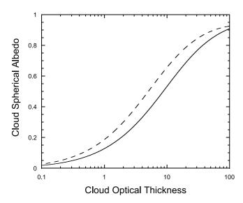
**Figure 2.** Examples of relationship between cloud spherical albedo and cloud optical thickness. Solid curve corresponds to a liquid water cloud layer composed of droplets with an effective radius of 11  $\mu$ m. Dashed curve corresponds to an ice cloud layer composed of inhomogeneous hexagonal crystals. Wavelength is  $\lambda = 865$  nm.
