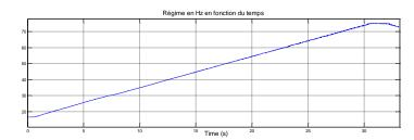
Fig. 8 The rotation speed of the diesel engine estimated from the tachometer signal
