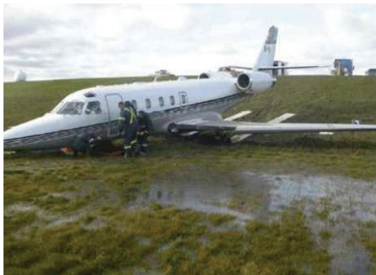
Figure 4: Example of Major/Hazardous runway excursion – Landing case [20]
