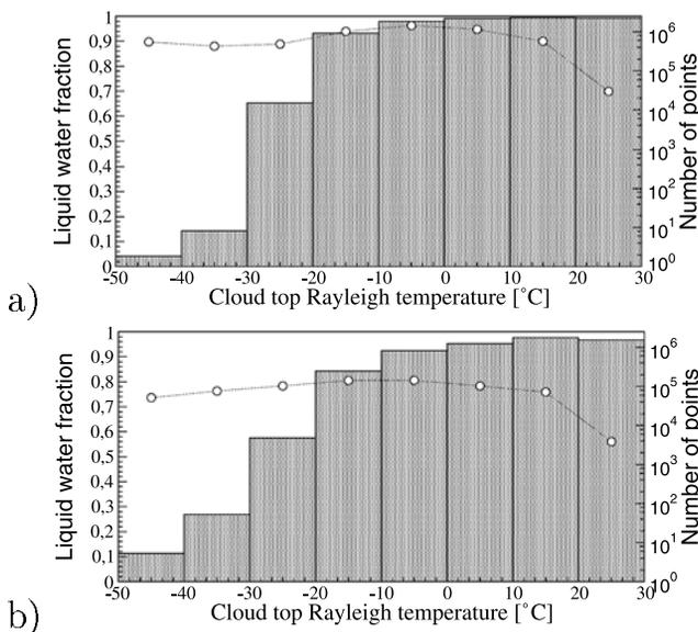
**Figure 2.** Fraction of liquid water at cloud top as a function of the cloud Rayleigh temperature in the POLDER observations at a) the POLDER resolution and b) the GCM resolution. The dashed line shows the number of points in each bin (right scale).
