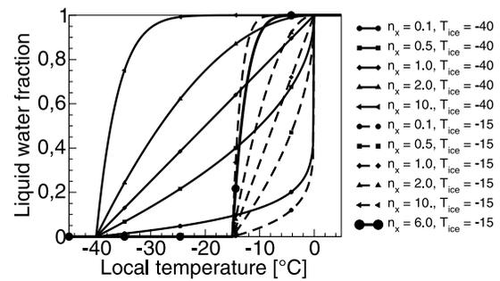
**Figure 1.** Liquid water fraction as a function of the local temperature for  $T_{ice} = -15^\circ\text{C}$  and  $T_{ice} = -40^\circ\text{C}$ , with values for  $n_x \in [0.1, 0.5, 1, 2, 10]$ . The bold line refers to the standard model parameters  $T_{ice} = -15^\circ\text{C}$  and  $n_x = 6$ .
