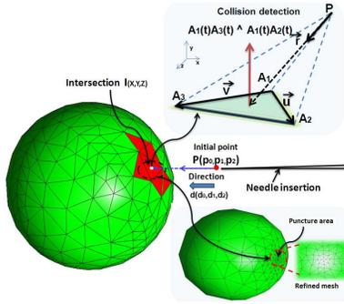
Fig. 7. Scheme illustrating the collision detection algorithm using a simple triangle points intersection problem: needle intersection with triangle surface of the cell, and the refining of the mesh.
