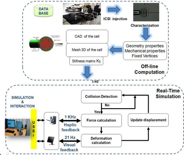
Fig. 6. Computational architecture for simulating force-reflecting deformable cell micro-injection in a virtual environment. The figure shows the two simulation phases used for the real-time micro-injection of the cell: (i) *off-line* pre-calculations of stiffness matrices and (ii) simulation of visual and haptic interaction.
