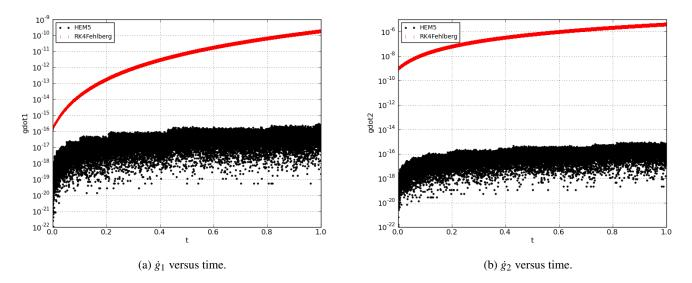
Fig. 3: Four bar linkage example. Drift of the constraints at the velocity level
