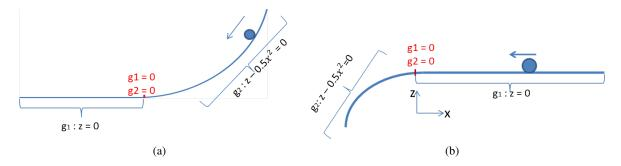
Fig. 7: Systems with geometrical discontinuities, illustrative examples
