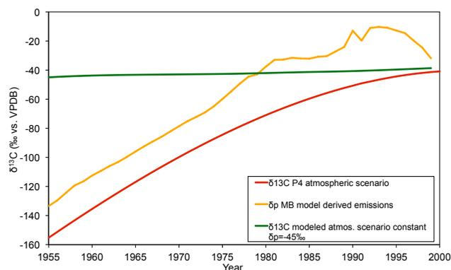
**Fig. 9.** Temporal evolution of reconstructed atmospheric  $\delta^{13}\text{C}$  values (‰, red, best fit 4th degree polynomial from firn air modeling) which are used as mass balance model input to calculate  $\delta^{13}\text{C}$  of the CFC-12 emissions ( $\delta_{\text{p}}$ , orange); mass balance calculated atmospheric scenario with constant  $\delta_{\text{p}} = -45\text{‰}$  and initial (1955)  $\delta$  of  $-45\text{‰}$  (green).
