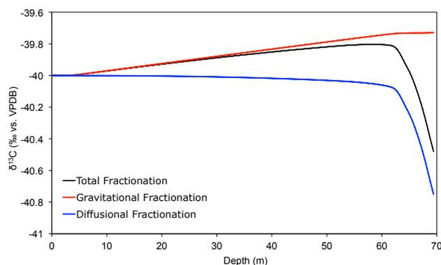
**Fig. 8.** CFC-12  $\delta^{13}\text{C}$  Modeled fractionation effects from gravitation (red) and diffusion (blue) and the sum thereof (black) based on a constant atmospheric  $\delta^{13}\text{C}$  ( $-40\text{‰}$ ) with time scenario input to the forward model.
