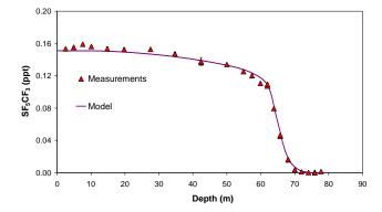
**Fig. 3.** The observed amounts (symbols) of SF<sub>5</sub>CF<sub>3</sub> in samples collected at different depths of firn at the NEEM drilling site, Greenland. The purple line is the result of taking the long-term trend of the gas in the atmospheric model domain box appropriate for NEEM, based on the best fit to Cape Grim (red line in Fig. 1), and used as input to the firn diffusion model.
