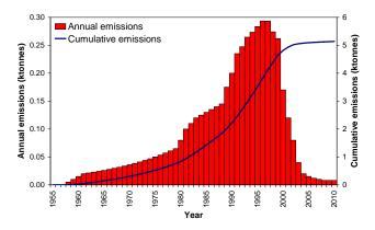
**Fig. 2.** The model-derived annual and cumulative emissions of SF<sub>5</sub>CF<sub>3</sub> used to produce the atmospheric model fit scenario presented in Fig. 1 (the red line in Fig. 1).
