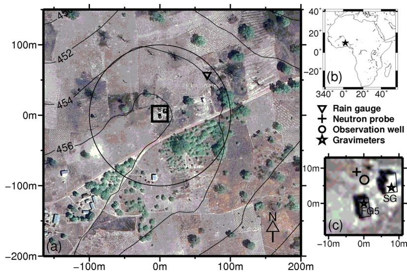
**Figure 1.** Study area, measurement settings: gravimeters (FG5 and SG) and their shelters. Neutron probe borehole and observation well are respectively located 9 and 7 m to the FG5 location. The circle shows the 100-m radius zone of influence for gravity variations at the FG5 site. *Google Earth* image, 2010 February 4.
