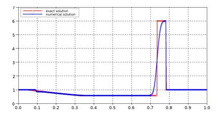
Fig. 6.6. A Riemann problem (Test 3 of [21, Chapter 4]) –  $\rho \sim u \sim e \sim p$  scheme – h = 0.001 and  $\delta t = h/100$  – Density at t = 0.012.
