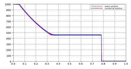
Fig. 6.2. A Riemann problem (Test 3 of [21, Chapter 4]) – h=0.001 and  $\delta t=h/100$  – Pressure at t=0.012.
