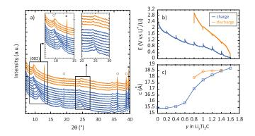
**Figure 2.** a) in-situ XRD patterns of  $Ti_2C$  collected each  $0.2 \, \text{Li}^+$  at a C/10 rate for charge (blue curves) and discharge (orange curves), \*: unreacted  $Ti_2AlC$ ,  $\circ$ : unreacted  $Ti_3AlC_2$ , b) corresponding constant current charge/discharge curve, and c) c parameter calculated from (002) peak shift during charge and discharge.
