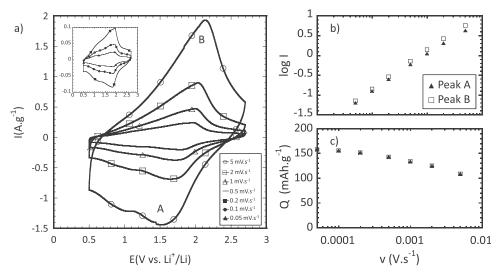
**Figure 4.** a) cyclic voltammetry curves from  $0.05 \text{ mV} \cdot \text{s}^{-1}$  to  $0.2 \text{ mV} \cdot \text{s}^{-1}$  (inset), and from  $0.5 \text{ mV} \cdot \text{s}^{-1}$  to  $5 \text{ mV} \cdot \text{s}^{-1}$ , b) plot of peak current (in A.g<sup>-1</sup>) as a function of the potential scan rate, and c) specific capacity as a function of scan rate.
