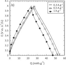
Figure 7. a) cyclic voltammetry curves at 5 mV · s<sup>-1</sup> of a YP17 activated carbon in 1M LiPF<sub>6</sub> EC:DMC (1:1) electrolyte with different voltage window, and b) constant current charge and discharge curves at 300 mA · g<sup>-1</sup>, 500 mA · g<sup>-1</sup>, and at 1 A · g<sup>-1</sup> between 3 V and 4 V vs. Li<sup>+</sup>/Li.
