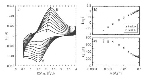
Figure 5. a) cyclic voltammetry curves obtained with a CME from  $5 \text{ mV} \cdot \text{s}^{-1}$  to  $100 \text{ mV} \cdot \text{s}^{-1}$ , b) plot of peak current (in mA) as a function of the potential scan rate, and c) capacity as function of the potential scan rate.
