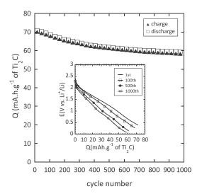
**Figure 9.** charge and discharge specific capacity vs. cycle number of a Ti<sub>2</sub>C/YP17 asymmetric cell at 10C charge and 10C discharge with no relaxation between cycles. The capacity is based on the Ti<sub>2</sub>C electrode. Inset: corresponding curves of Ti<sub>2</sub>C electrode at different cycles showing the potential drift of the negative electrode.
