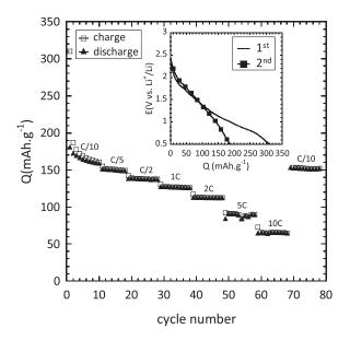
Figure 3. charge and discharge specific capacities of  $Ti_2C$  from C/10 to 10C rate. Inset shows the capacity loss between the  $1^{st}$  and  $2^{nd}$  galvanostatic charges.
