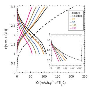
**Figure 8.** three-electrode constant current charge and discharge curves of a Ti<sub>2</sub>C/YP17 asymmetric cell cycled between 3.5 V and 1.0 V from 1C to 20C rate. Specific capacity is represented based on the Ti<sub>2</sub>C electrode. Inset: corresponding curves of the Ti<sub>2</sub>C electrode.
