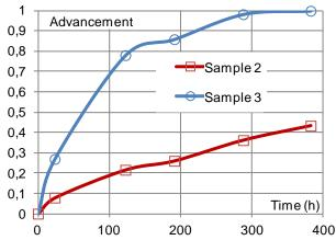
Figure 5: Advancement vs. time for the hydration of sample 2 (small grains) and sample 3 (large grains).
