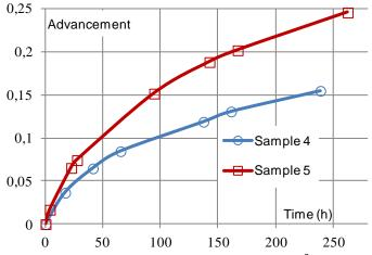
**Figure 6:** Advancement vs. time for the hydration of sample 4 (507 kWh.m<sup>-3</sup>, with vermiculite) and sample 5 (577 kWh.m<sup>-3</sup>, without vermiculite).
