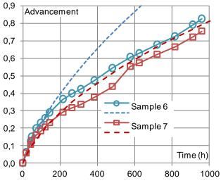
**Figure 11:** Advancement vs. time for hydrations for samples 6 (with gas diffuser) and 7 (without diffuser): experimental results (symbols) and simulations using the sharp front model (dotted line).
