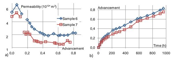
**Figure 8:** Samples 6 (with gas diffuser) and 7 (without diffuser) a) Permeability vs. advancement and b) advancement vs. time during hydration.
