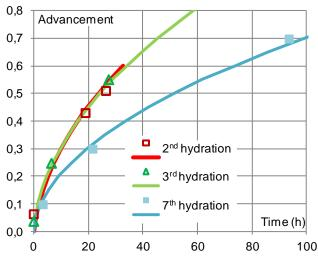
**Figure 10:** Advancement vs. time for hydrations 2, 3 and 7 of sample 1: experimental results (symbols) and simulations using the sharp front model (line).
