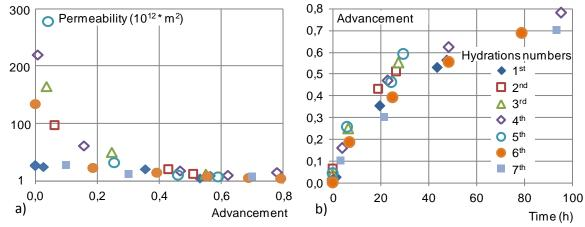
**Figure 3:** Experimental hydrations of sample 1: a) permeability k vs. reaction advancement and b) advancement vs. time for seven hydrations
