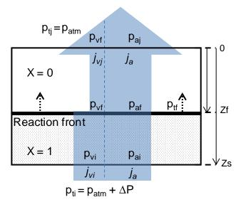
Figure 9: Schematic representation of the porous bed of reactive salt, crossed by a flow of moist air.
