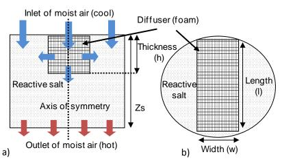
**Figure 7:** Diagram of a sample of salt bed with a diffuser (size: 98.9 mm x 22.3 mm x 31.4 mm). a) Vertical sectional view (along the symmetry axis of the sample), b) top view of the sample.
