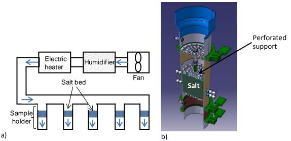
**Figure 2:** Experimental set-up for mass transfer and kinetics characterizations a) the experimental bench, b) the sample holder.
