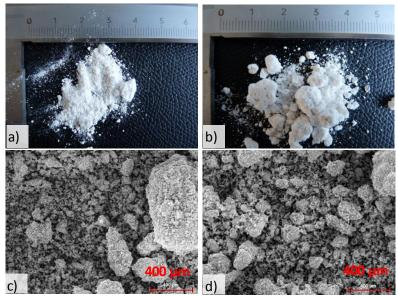
**Figure 4:** Photographies of a) sample 2 b) sample 3. Pictures with a scanning electron microscopy (SEM) of c) sample 2, d) sample 3.
