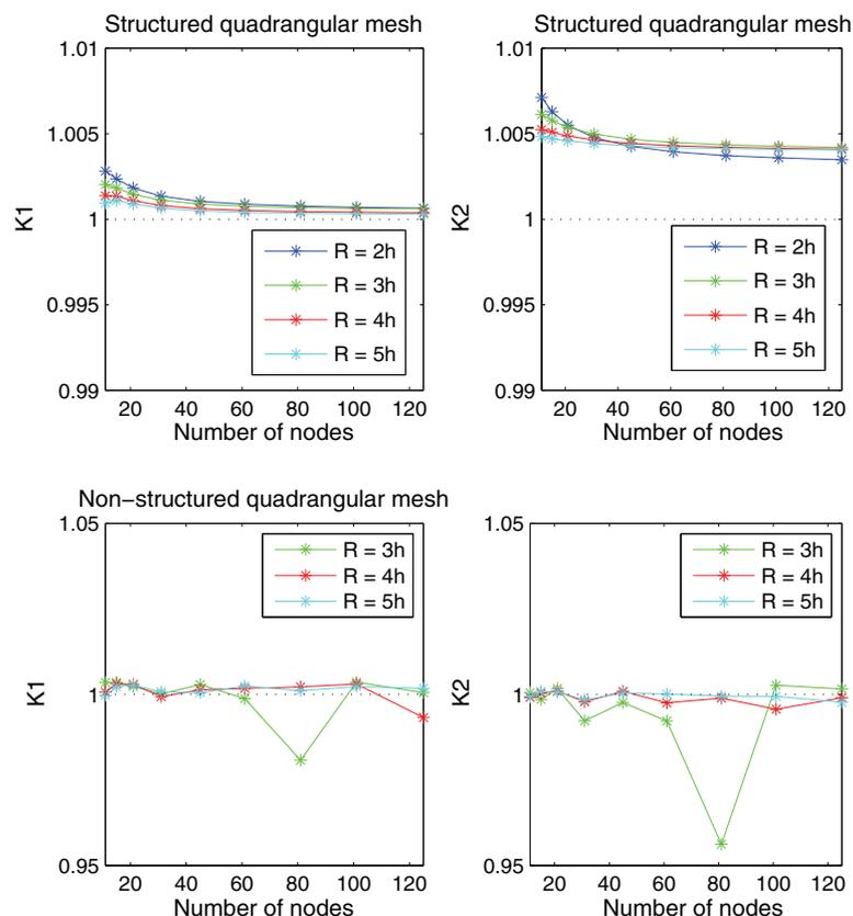
Figure 11. Stress intensity factors calculations—Direct estimate—First test case—Quadrangular meshes.
