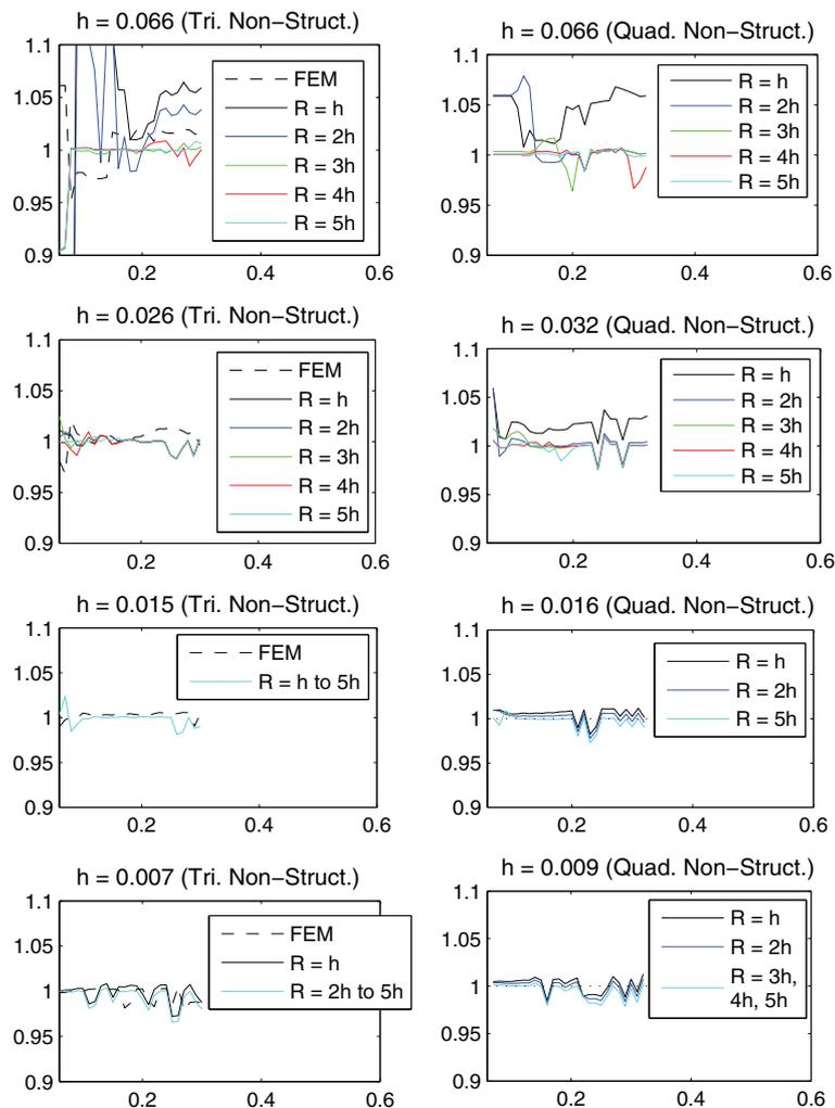
Figure 15. Normalized  $K_1$  versus  $\mathcal{R}_J$ —J-integral—First test case.
