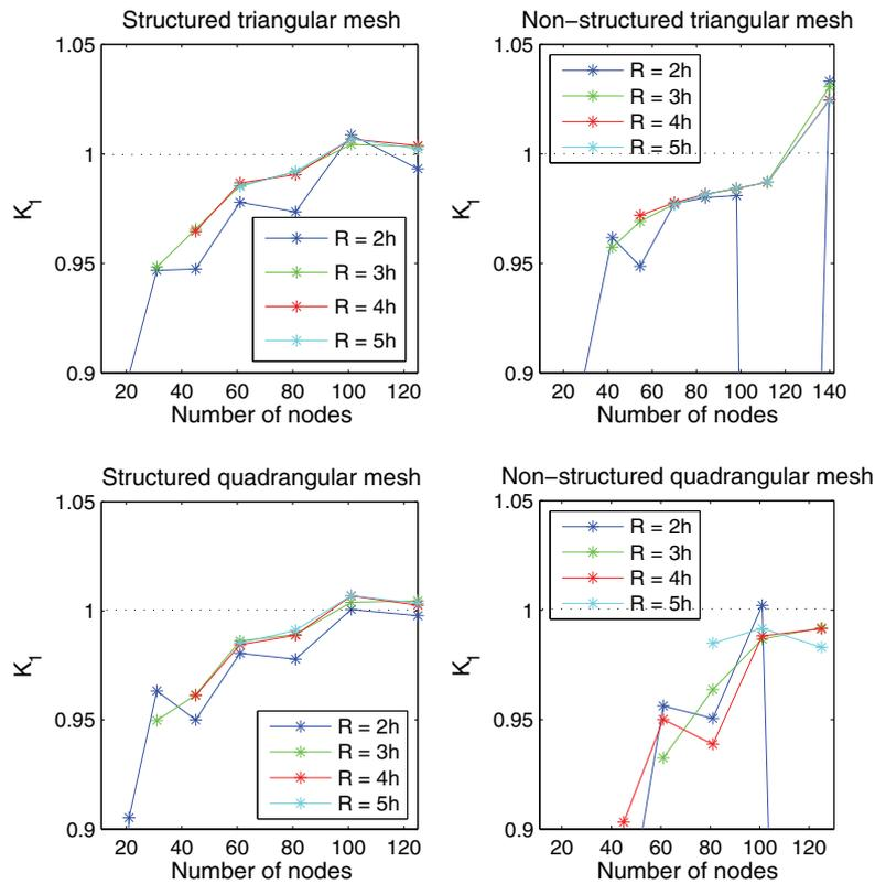
Figure 12. Stress intensity factors calculations—Direct estimate—Second test case.
