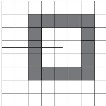
Figure 8. Ring of elements enclosing the crack tip.
