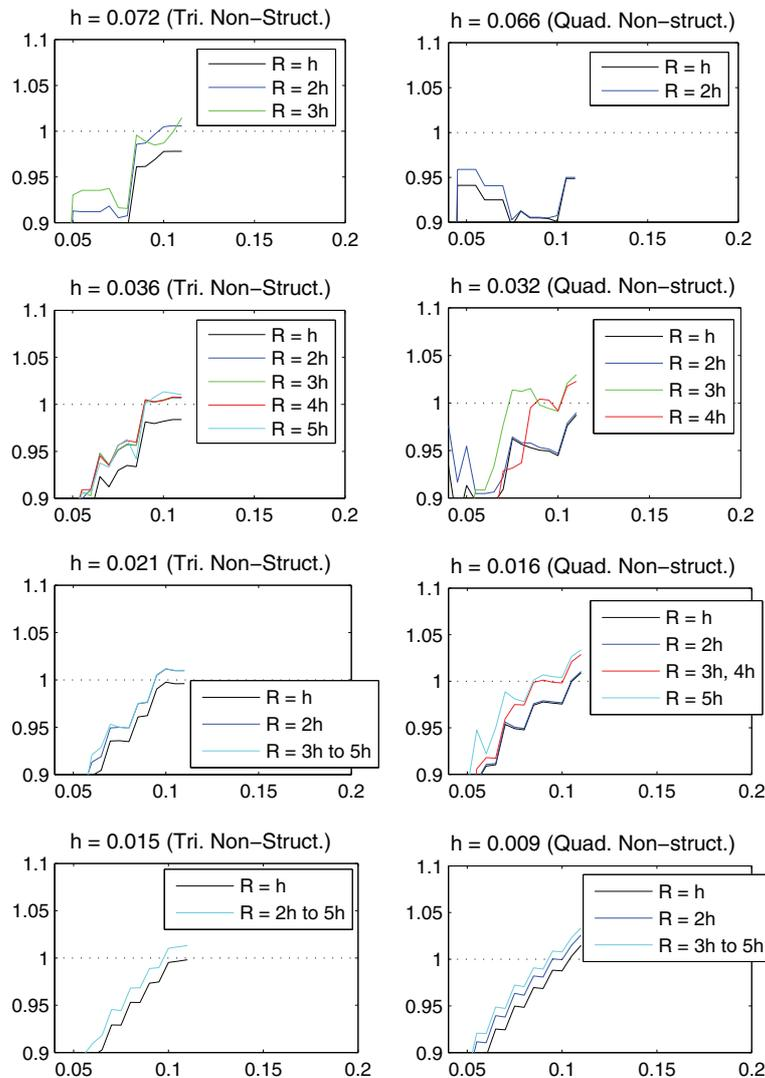
Figure 16. Normalized  $K_1$  versus  $\mathcal{R}_J$ —J-integral—Second test case.
