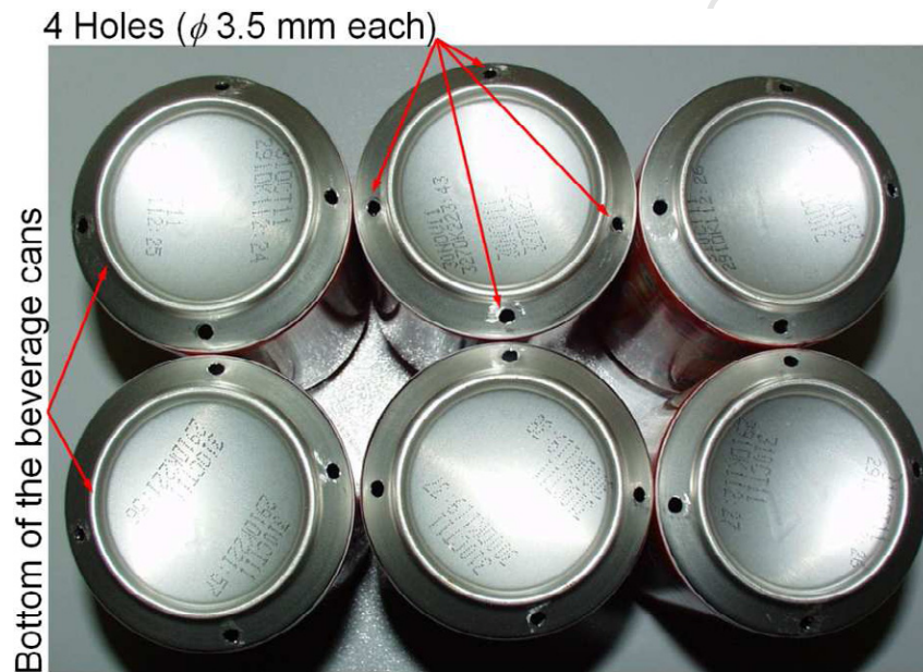
Figure 15: Beverage cans with holes at the bottom (to remove the air inside the beverage can during the crushing process).
