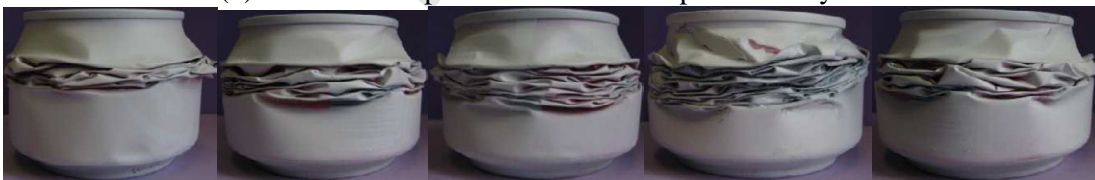
(e) Deformation patterns for initial impact velocity 4.4 m/s
