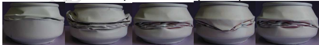
(f) Deformation patterns for initial impact velocity 4.9 m/s
