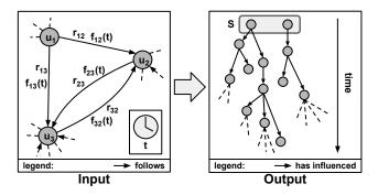
Figure 3: The T-BaSIC model predicts the diffusion process along a continuous time-axis based on the time-delay and diffusion function on each arc, starting from a set S of initially activated nodes.
