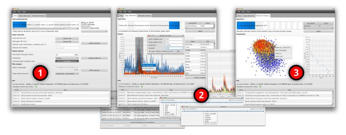
Figure 5: Illustration of the different services offered by SONDY, from left to right: (1) the data manipulation service, (2) the topics and trends exploration service and (3) the network analysis service.
