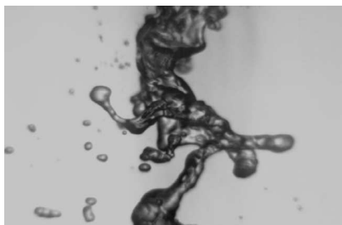
Figure 1. An example of atomized slow liquid flow by a rapid air stream
