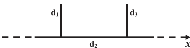
FIG. 1. Schematic illustration of the one-dimensional electromagnetic waveguide of length d_2 with dangling resonators on both sides. The whole structure is inserted between two semi-infinite waveguides. The lengths of the dangling resonators are d_1 and d_3 .
