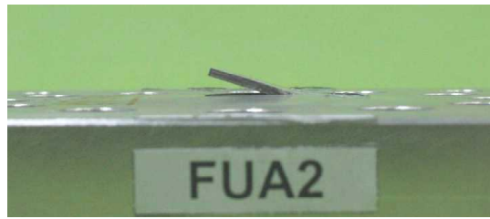
(a) Experimental deflection, \alpha \sim 20^\circ
