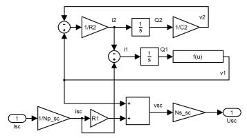
Fig. 3. Matlab simulation model of Supercapacitors pack
