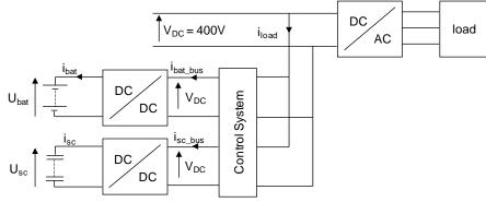
Fig. 10. Topology of the controlled SC's/battery combination
