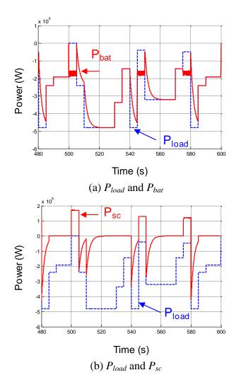
Fig. 22. Power waveforms with intermediary SC's recharging
