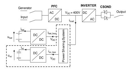
Fig. 1. Topology of the 500 kVA UPS
