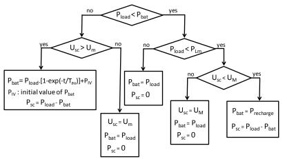
Fig. 12. Chart of the SC's/battery combination system
