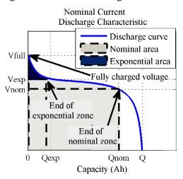
Fig. 5. Typical discharge curve [33]
