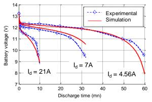
Fig. 6. Experimental and simulated battery discharge curves
