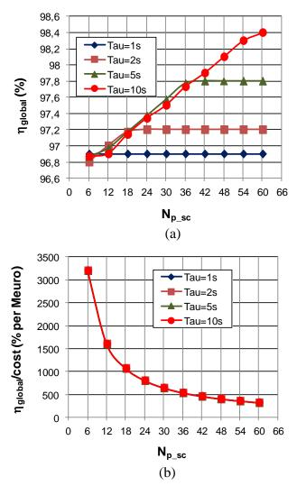
Fig. 18. Energy efficiency versus  $T_{au}$  and  $N_{p_{sc}}$
