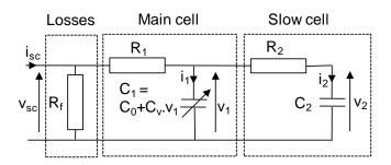
Fig. 2. Supercapacitor simplified circuit: two branches model
