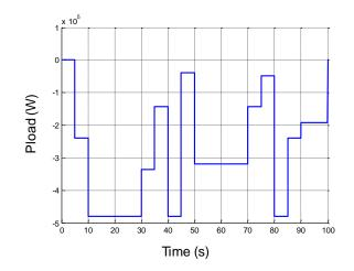
Fig. 13. Typical harmonic load power of an UPS
