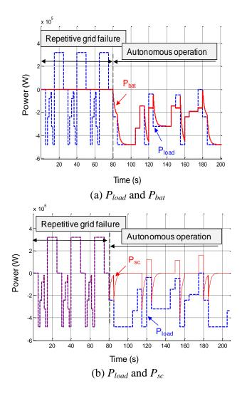
Fig. 23. Power waveforms for successive brownout and autonomous operation
