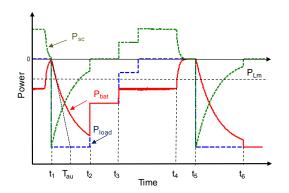
Fig. 11: Principle of power sharing between SC's and the battery
