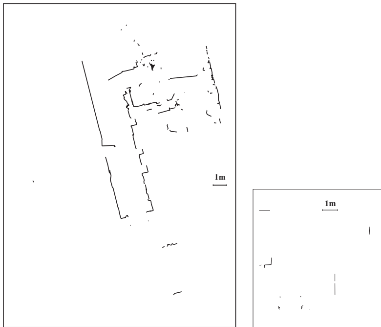
Fig. 5. The final map obtained with the sequential method (left) and partial map S_{21} (right).
