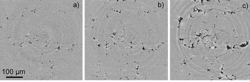
Fig. 1. Damage evolution on slice no. 56 (Fig. 2) having the highest void area fraction in the last reconstructed state of the sample deformed at 773 K. (a)  $t = 0.36 t_f$ , (b)  $t = 0.53 t_f$  and (c)  $t = 0.79 t_f$ . The creep time is indicated as part of the failure time  $t_f$ .
