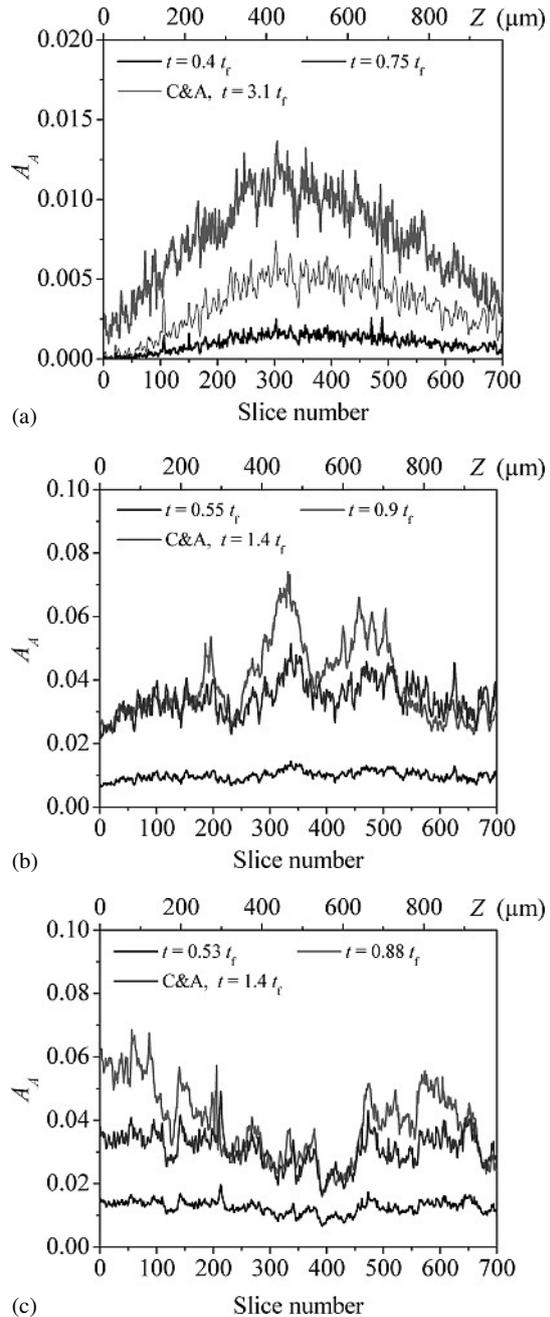
Fig. 6. Comparison between experimentally determined and predicted distributions of void area fraction along the gauge length. The experimental distributions correspond to the final reconstructed state (F) and a previous reference state (R) with a cross-correlation coefficient larger than 0.7. The reference state has been used as input for prediction of damage distribution according to the model of Cocks and Ashby [7]. (a) sample deformed at 573 K, (b) at 723 K and (c) at 773 K.
