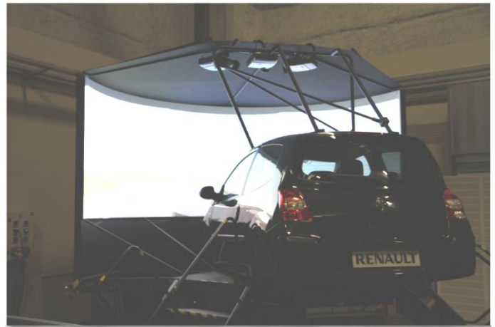
Figure 17. Operating of the dynamic driving simulator SAAM
