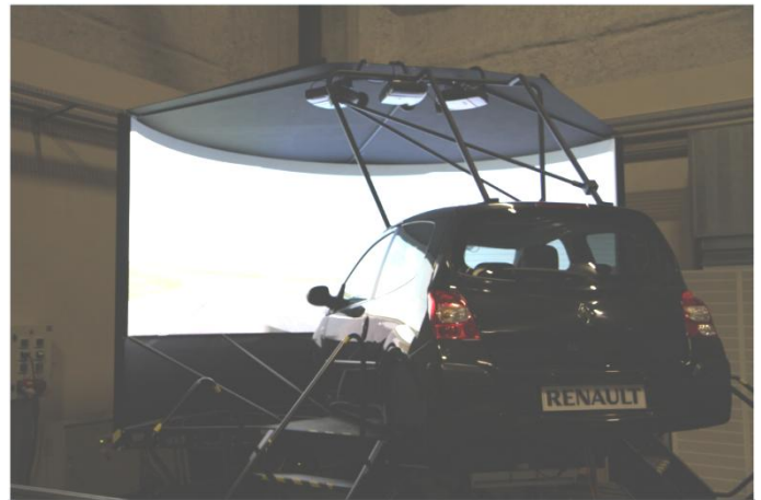
Figure 17. Operating of the dynamic driving simulator SAAM
