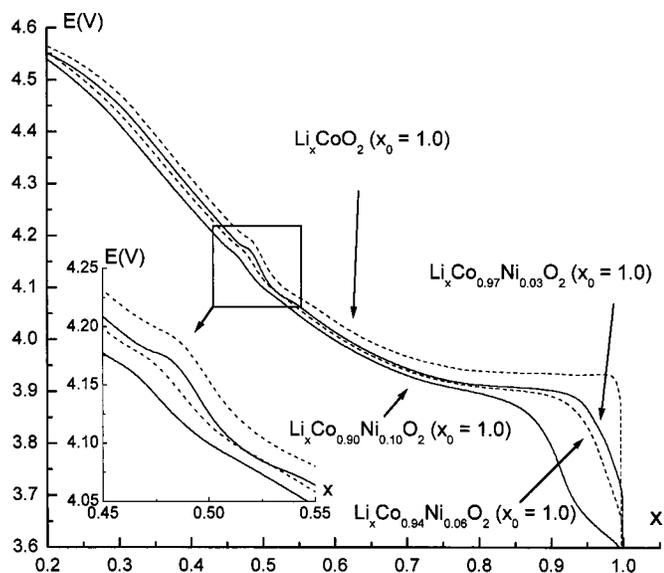
**Figure 2.** First galvanostatic charge of  $\text{Li}/\text{Li}_x\text{Co}_{1-y}\text{Ni}_y\text{O}_2$  ( $x_0 = 1.0$ ,  $y = 0.0, 0.03, 0.06$ , and  $0.10$ ) electrochemical cells ( $J = 100 \mu\text{A cm}^{-2}$ ;  $m_{\text{Li}(\text{CoNi})\text{O}_2} = 30 \text{ mg}$ ).
