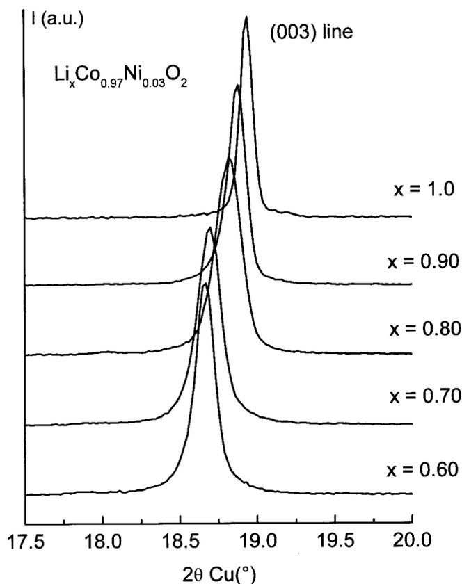
**Figure 4.** Expansion of the (003) Bragg reflection of the XRD patterns of the electrochemically deintercalated  $\text{Li}_x\text{Co}_{0.97}\text{Ni}_{0.03}\text{O}_2$  ( $x_0 = 1.0$ ) samples ( $0.60 \leq x \leq 1.0$ ).
