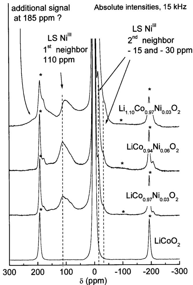
**Figure 8.** 15 kHz  $^7\text{Li}$  MAS NMR spectra for the various  $\text{Li}_{x_0}\text{Co}_{1-y}\text{Ni}_y\text{O}_2$  phases ( $x_0 = 1.0, 1.10$ ;  $y = 0.0, 0.03, 0.06$ ), (\* = spinning side bands).
