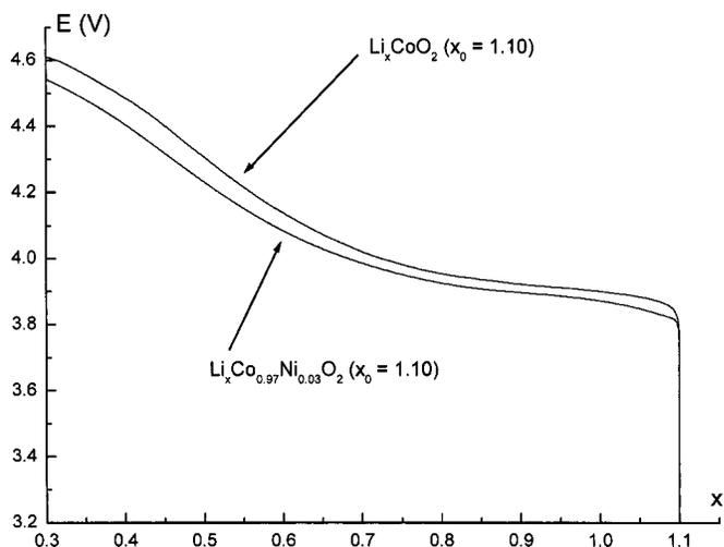
**Figure 5.** First galvanostatic charge of  $\text{Li}/\text{Li}_x\text{Co}_{1-y}\text{Ni}_y\text{O}_2$  ( $x_0 = 1.10$ ,  $y = 0.0, 0.03$ ) electrochemical cells ( $J = 100 \mu\text{A cm}^{-2}$ ;  $m_{\text{Li}(\text{Co,Ni})\text{O}_2} = 30 \text{ mg}$ ).
