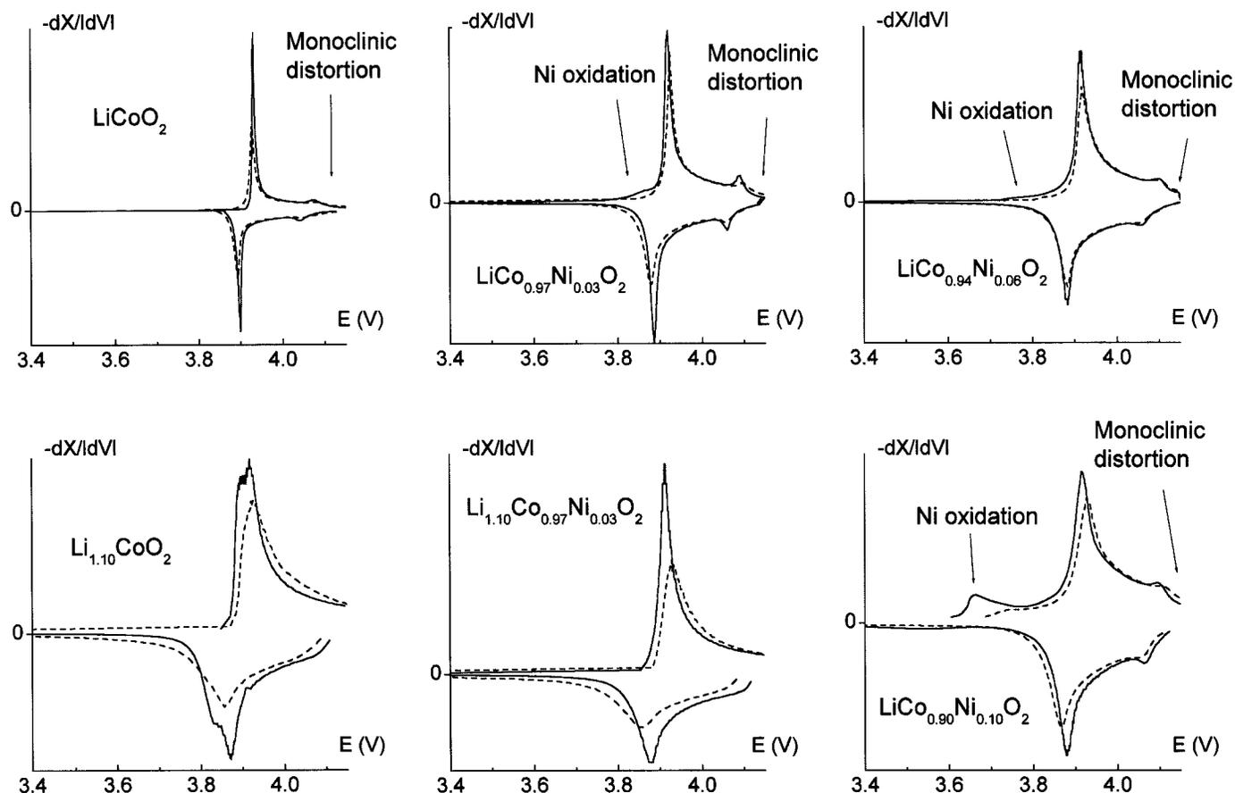
**Figure 7.**  $-dx/dV = f(V)$  derivatives curves of the first (solid line) and 10th (dashed line) cycles of the various  $\text{Li}/\text{Li}_x\text{Co}_{1-y}\text{Ni}_y\text{O}_2$  ( $x_0 = 1.0, 1.10$ ;  $y = 0.0, 0.03, 0.06, \text{ and } 0.10$ ) electrochemical cells ( $J = 400 \mu\text{A cm}^{-2}$ ;  $m_{\text{Li}(\text{CoNi})\text{O}_2} = 15 \text{ mg}$ ) between 2.7 and 4.15 V.
