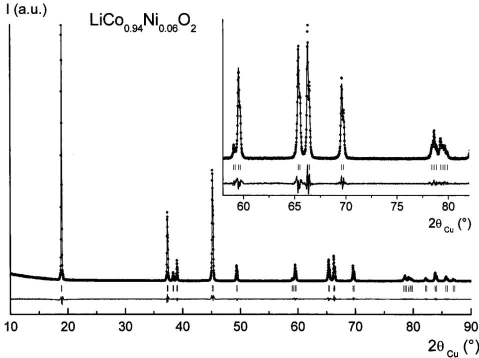
**Figure 1.** Observed and calculated XRD profiles for  $\text{Li}_{1.0}\text{Co}_{0.94}\text{Ni}_{0.06}\text{O}_2$ . filled circles: observed; solid line, calculated; lower trace, difference plot; bars, reflections.
