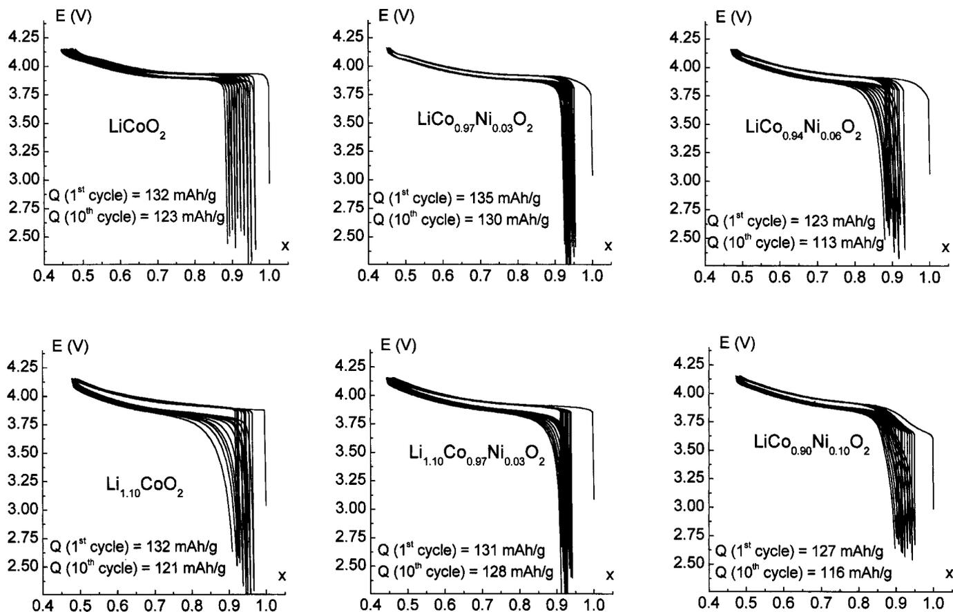
**Figure 6.** Cycling behavior of the various  $\text{Li}/\text{Li}_x\text{Co}_{1-y}\text{Ni}_y\text{O}_2$  ( $x_0 = 1.0, 1.10$ ;  $y = 0.0, 0.03, 0.06$ , and  $0.10$ ) electrochemical cells ( $J = 400 \mu\text{A cm}^{-2}$ ;  $m_{\text{Li}(\text{Co,Ni})\text{O}_2} = 15 \text{ mg}$ ,  $C/20$  rate) between 2.7 and 4.15 V.
