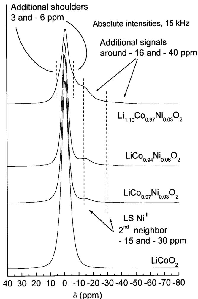
**Figure 9.** Expansion of the central signal of 15 kHz  $^7\text{Li}$  MAS NMR spectra for the various  $\text{Li}_{x_0}\text{Co}_{1-y}\text{Ni}_y\text{O}_2$  phases ( $x_0 = 1.0, 1.10$ ;  $y = 0.0, 0.03, 0.06$ ).
