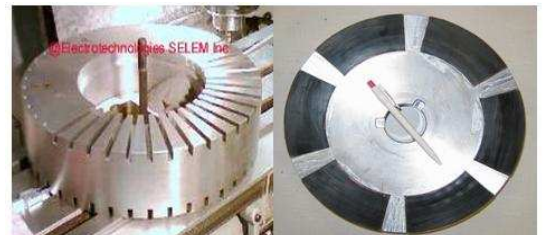
Fig. 2. Stator and rotor of the proposed machine.
