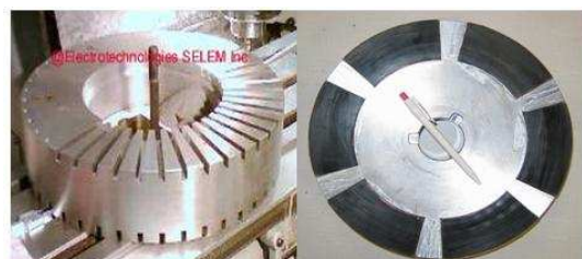
Fig. 2. Stator and rotor of the proposed machine.
