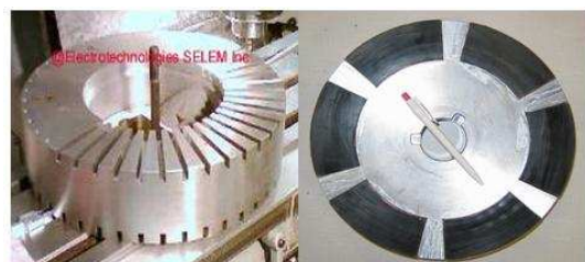
Fig. 2. Stator and rotor of the proposed machine.
