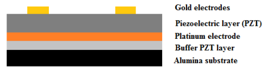
Figure 1: Schematic representation of thick-film structure.
