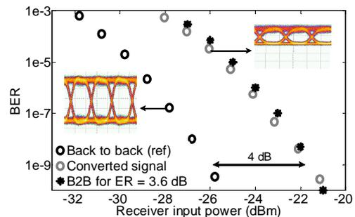
**Fig. 4:** BER curves of the converted signal.
