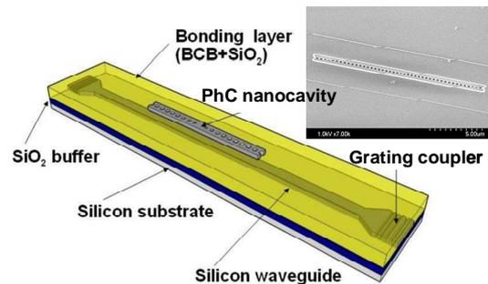
**Fig. 1:** Device principle. SEM picture in the inset.
