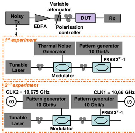
Fig. 5: Experimental setup for the noise limiter.
