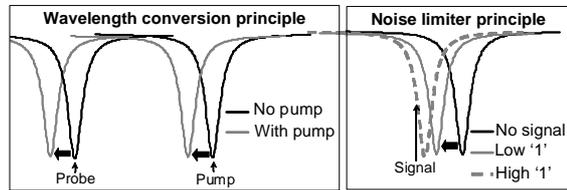
**Fig. 3:** Principle of wavelength conversion and power limiter.
