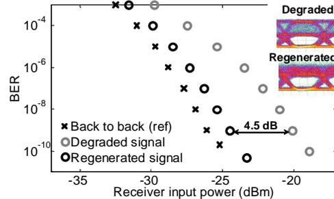
Fig. 7: BER curves of the noise limiter.
