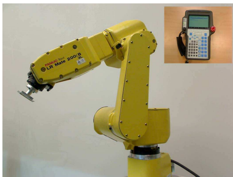
Figure 2 LRMate 200iB Robot.
