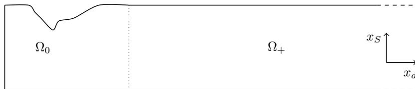
Figure 1: A realization of the domain  $\Omega$  in two dimensions, representing a waveguide of semi-infinite length with a local boundary deformation.
