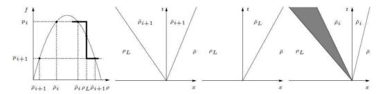
FIGURE 4. With reference to Example 2, the flux configuration and three different solutions  $\rho_1$ ,  $\rho_2$  and  $\rho_3$  to the same Riemann problem are represented from left to right. Here  $\check{\rho}_L = \check{\rho}(f(\rho_L))$ .
